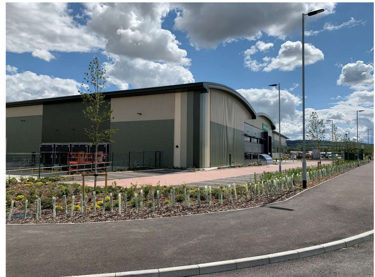
Fig 36. Column mounted and building mounted, light fittings for the development plots and highways.
